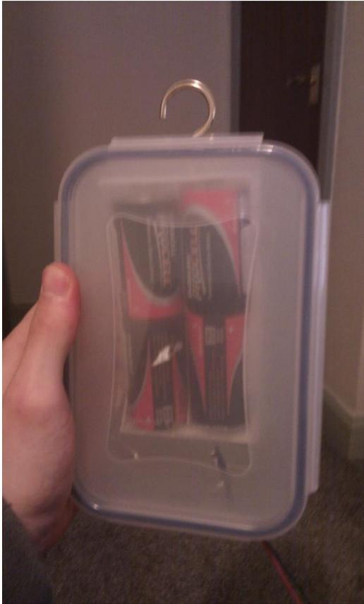
**Figure 8.** Water resistant battery pack container.
